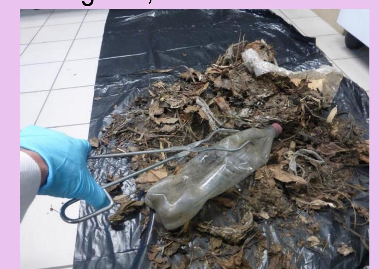
100L of runoff water are collected upstream of the grid refusals during rain events for microplastic analysis. This water is then filtered with a 80 µm net and microplastics are analyzed.
