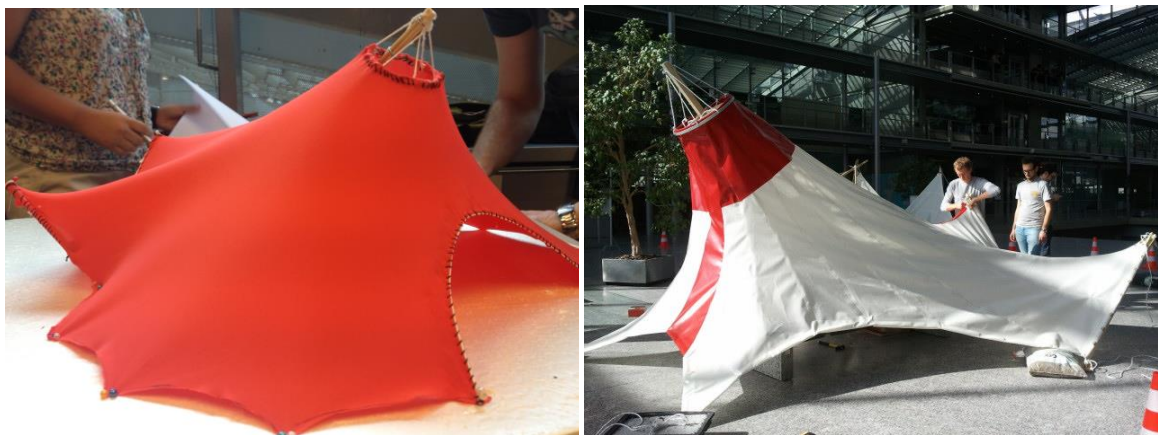
Figure 3: “El para  so de la siesta”: Lycra model and final structure (photo by courtesy C. Douthe)
