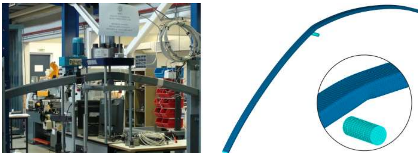
Figure 23: High arches' deformed shape under tension loading, at the end of the test (left) and the GMNA (right)
