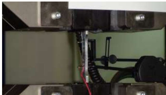
Figure 5: Tensile coupon test.
