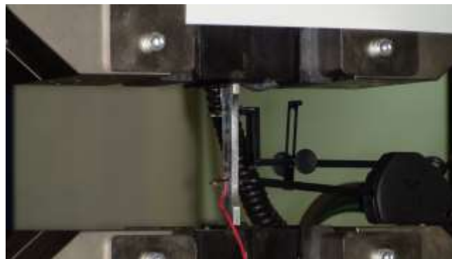
Figure 5: Tensile coupon test.
