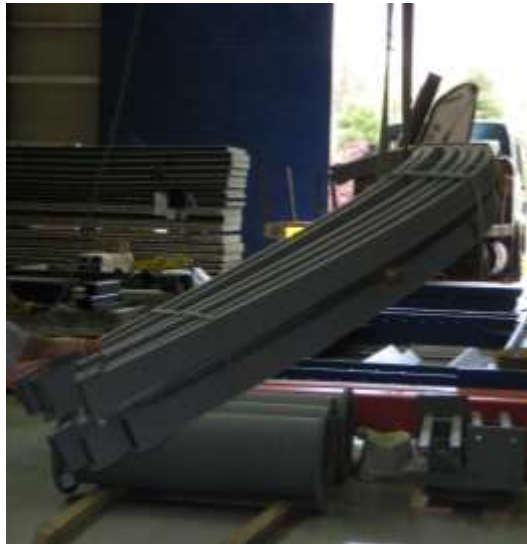
Figure 3: Twelve circular steel arches received for testing at the Institute of Steel Structures of NTUA.
