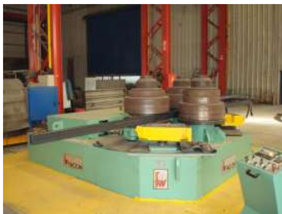
Figure 1: Roller bending machine for constructional steel.
