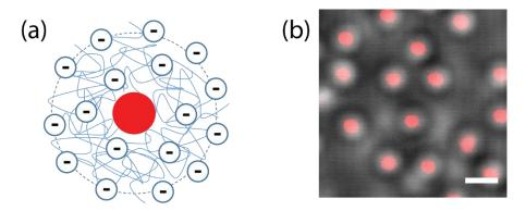
Figure 1: (a) Schematic of a microgel particle composed of a rigid fluorescent core (160 nm) and a pNIPAM structure with negative charges at pH>4.25 (pKa of acrylic acid is 4.25). Charges are throughout the structure; polymer chains extend at the surface. (b) Image of a microgel suspension (superposition of fluorescent and bright field images). The scale bar is 1  $\mu$ m.
