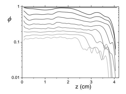
Figure 9: Drying of bead packing filled with silica particle suspensions at  $\psi_0 = 10\%$ . Water saturation profiles every 10 hours after the beginning. The black line is the initial saturation.
