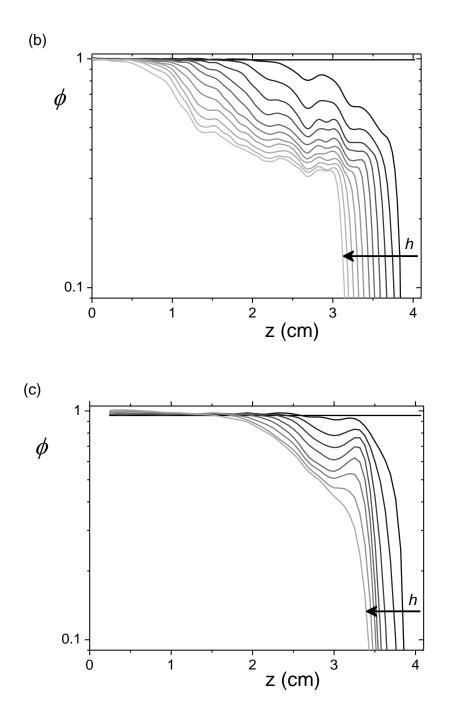
Figure 8: Drying of bead packing filled with microgel suspensions: (a)  $c_0 = 3.5$  g/L, (b)  $c_0 = 10.4$  g/L, (c)  $c_0 = 45.1$  g/L. Water saturation profiles every 10 hours after the beginning. The black line is the initial saturation.
