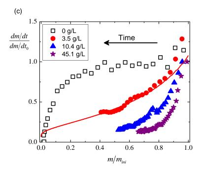
Figure 5: Drying of microgel suspensions in bead packing for different concentrations: pure water (squares),  $c_0 = 3.5$  g/L (red circles), 10.4 g/L (blue triangles), 45.1 g/L (purple stars) and 33% (orange diamonds). Water mass loss as a function of time, in linear (a) and logarithmic scale (b). Drying rate normalized by initial value as a function of normalized water mass (c). The red continuous line corresponds to the migration-diffusion model for soft particles with  $c_0 = 3.5$  g/L.
