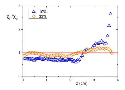
Figure 12: Drying of bead packing filled with silica suspensions: 10% (blue triangles) and 33% (orange diamonds). Final particle distribution  $\chi_f$  normalized by the initial one  $\chi_0$ . The red line is the initial homogeneous state.
