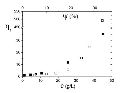
*Figure 2:* Relative viscosity of **silica suspension in water (open squares)** as a function of the volume concentration of particles (top abscissa), and **of microgel suspension (filled squares)** as a function of the microgel mass concentration (bottom abscissa).
