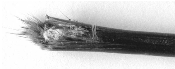
(b) Creep rupture in torsion-bending
