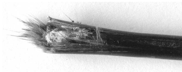
(b) Creep rupture in torsion-bending
