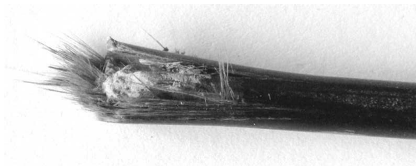
(b) Creep rupture in torsion-bending
