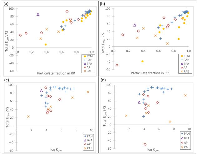
Figure 8: Relationships between total median concentration reduction ( $E_{c50}$ ) and median particulate fraction ( $F_{p50}$ ) in (a) the vegetative filter strip, VFS and (b) the biofiltration swale, BFS and between total  $E_{c50}$  and octanol water partition coefficient ( $K_{ow}$ ) in (c) VFS and (d) BFS
