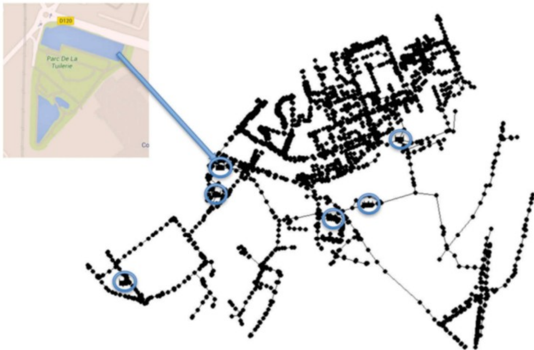
Figure 6. SWMM file of the Massy sub-catchment and the six storage basins, with the Cora basin (measurement point) highlighted.
