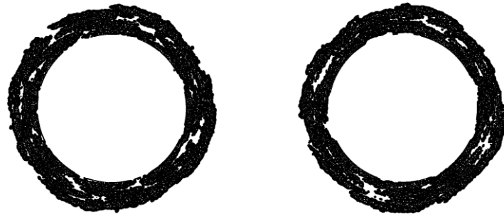
Fig.4 Cross-sectional slices at the two ends of the tube in the unit cell optimized for the FFT simulation.
