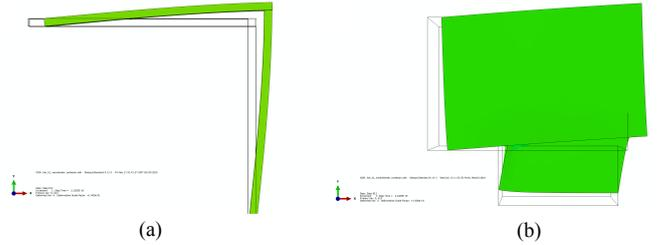
Figure 7: FE unit-cell under in-plane shear loading [1] for two limit cases: (a) slender beam regime at wide gaps ( $K_\theta \gg 1/\alpha_n$ ) and (b) rotational spring regime at narrow gaps ( $K_\theta \ll 1/\alpha_n$ )
