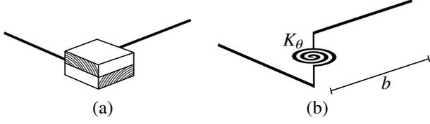
Figure 4: Wooden blocks connecting beams modeled as rotational spring deformable under in-plane rotation
