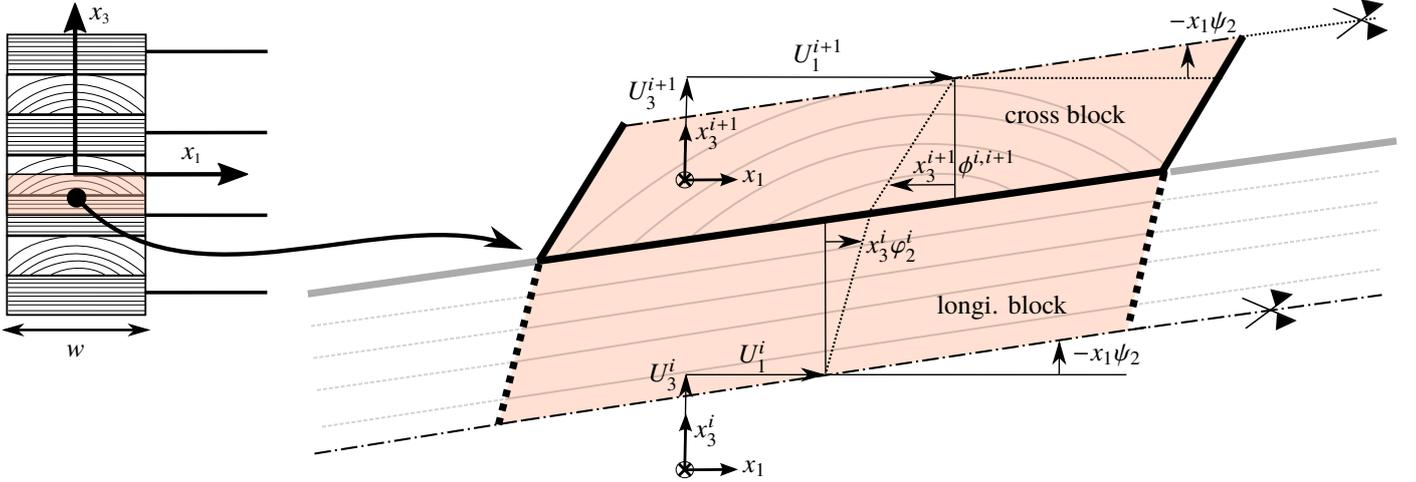
Figure 8: Out-of-plane shear kinematics in plane  $x_2 = 0$  of the thick interface between lamellae ( $\psi_2 < 0$ )
