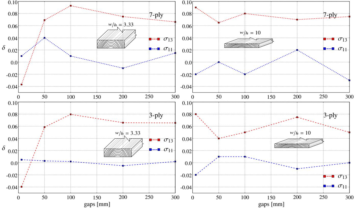
Figure 15: Relative difference  $\delta$  between numerical and closed-form maximum longitudinal and rolling shear stresses in 7-ply (top) and 3-ply (bottom) panels for  $w/h = 3.33$  (left) and  $w/h = 10$  (right)
