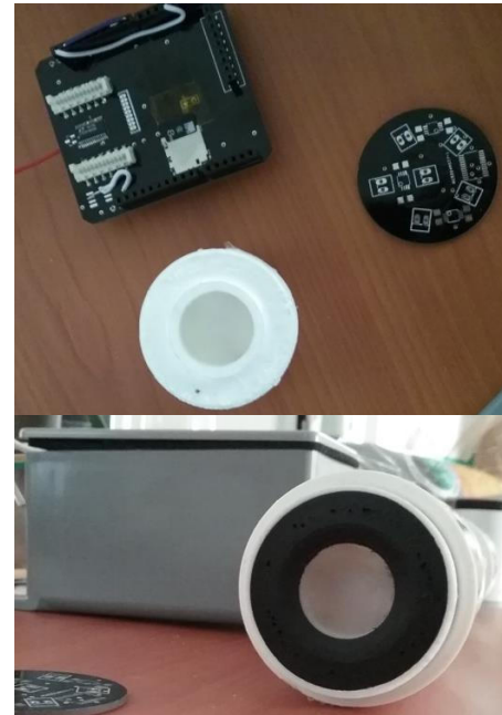
Fig. 3. Components and assembled optical sensor.
