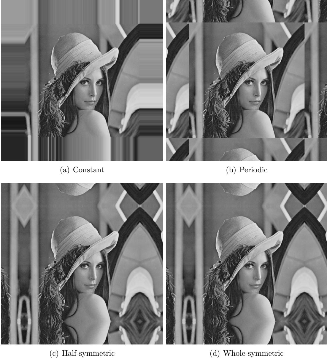
Figure 3: Extended image used during the prefiltering using Algorithm 4 for \varepsilon = 10^{-8} i.e. 8 digits and n = 11 . The image is extended of L_0^{(n,\varepsilon')} = 125 pixels from its boundary.
