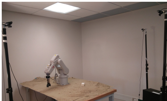
Fig. 5 Acquisition of real images to create our test dataset, with 3 cameras at arbitrary and varying positions
