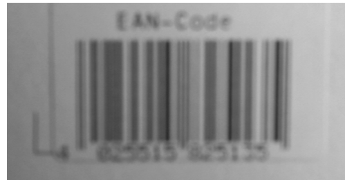
Fig. 1. A real barcode image with blur, noise and non uniform illumination
