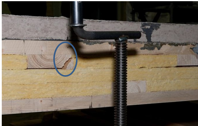
Figure 5 : Transverse shear cracking (blue circle) between layers 2 and 3 in a transverse wooden strip.
