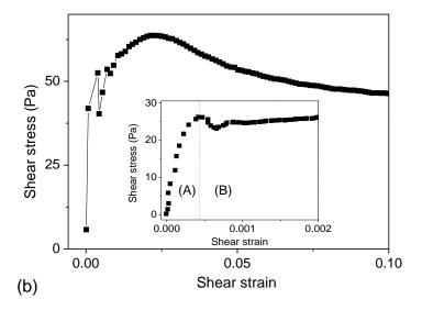
**Figure 3:** Shear stress as a function of shear strain during a creep test at high shear rate  $(10^{-2} \text{ s}^{-1})$  or low shear rate  $(3.10^{-4} \text{ s}^{-1})$  (inset) for: (a) a lime paste (water to lime ratio of 1.3) after 20 min. of rest, and (b) a cement paste (water to cement ratio of 0.4) after 2 min of rest. The vertical dotted line in the inset shows the position of the transition between the first and the second structure (see text).
