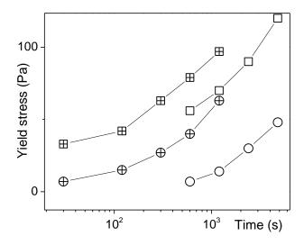
**Figure 5:** Critical stress associated with the transition between the first and second structure (circles) and stress peak (squares) for data of Figure 3 with a lime paste (open symbols) and a cement paste (crossed symbols).
