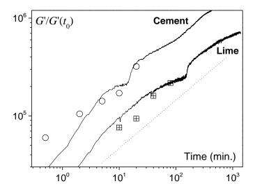
**Figure 8**: Elastic modulus in time measured from dynamic tests (continuous lines) at a frequency of 0.5Hz and comparison with data from creep tests at low shear rate  $(3.10^{-4} \text{ s}^{-1})$  for a lime paste ( $\phi = 28\%$ , crossed squares) and a cement paste ( $\phi = 44\%$ , circles). The dotted line of slope 1/2 is a guide for the eye.
