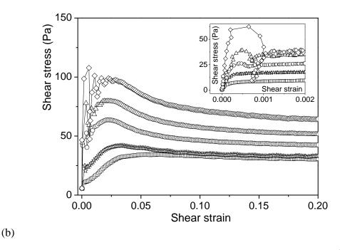
**Figure 4**: Shear stress as a function of shear strain during creep tests at high shear rate  $(10^{-2} \text{ s}^{-1})$  or low shear rate  $(3.10^{-4} \text{ s}^{-1})$  (inset) for (a) a lime paste (water to lime ratio of 1.3), and (b) a cement paste (water to cement ratio of 0.4) after different times of rest following preshear (from bottom to top): (lime) 10, 20, 40, and 80 min., (cement), 30 s, 2, 5, 10, and 20 min.
