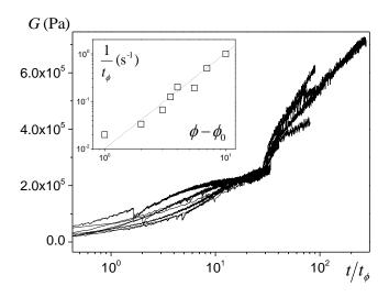
**Figure 10**: Elastic modulus for lime pastes at different solid volume fractions (data of Figure 9) as a function of the time rescaled by the characteristic time  $t_{\phi}$  (see text). The inset shows the variation of this parameter with the solid fraction. The dotted line in the inset has a slope  $\frac{1}{2}$ .
