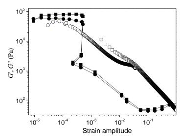
**Figure 7**: Elastic (filled symbols) and loss (open symbols) moduli measured as a function of strain amplitude (frequency 1 Hz) for a lime paste ( $\phi = 28\%$ ) (two tests on different samples of the same material (squares and circles)).
