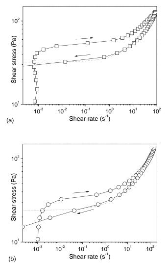
**Figure 2:** Apparent flow curve obtained from a shear rate sweep for: (a) a lime paste immediately after preparation with a water to lime ratio of 1.17; (b) a cement paste with a water to cement ratio of 0.4 by weight. The dotted line corresponds to a Herschel-Bulkley model fitted to data for the
