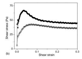
**Figure 6:** Shear stress as a function of shear strain during creep tests at high shear rate  $(10^{-2} \text{ s}^{-1})$  for: (a) a lime paste (water to lime ratio of 1.3) 20 min. after preshear following preparation (filled squares), and for the same test 1 h after the first one; (b) a cement paste (water to cement ratio of 0.4) 5 min. after preshear following preparation (filled squares), and for the same test 40 min. after the first one.
