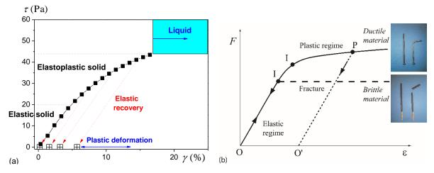
**Figure 2**: Stress vs final deformation from creep tests for (a) a typical YSF (here an emulsion, data from Maimouni et al 2016) and (b) typical solids (brittle or ductile).
