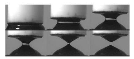
Figure 8: Successive views of a YSF shape during a traction test. [Courtesy Jalila Boujlel]
