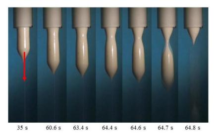
**Figure 7**: Successive views of a mayonnaise sample at different times during extrusion. The initial time (0 s) corresponds to the separation of the previous extrudate. [Figure 1 of Coussot and Gaulard 2005].
