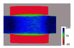
**Figure 4**: Flow of a yield stress fluid (concentrated emulsion with  $\tau_c$  =74 Pa) through a sudden enlargement (diameter 7 cm) then contraction (back to 3.5 cm diameter). Velocity map in a longitudinal cross-section for a mean velocity in the small conduit of 0.16 mm/s. The velocity amplitude (in microns per second) in each voxel is represented
