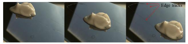
**Figure 3**: Successive views of a heap of emulsion (yield stress: 40 Pa) put on a smooth surface, at times: (a) 0, (b) 15.6 s, (c) 26 s. The sample length is about 3 cm. [Courtesy Xiao Zhang]
