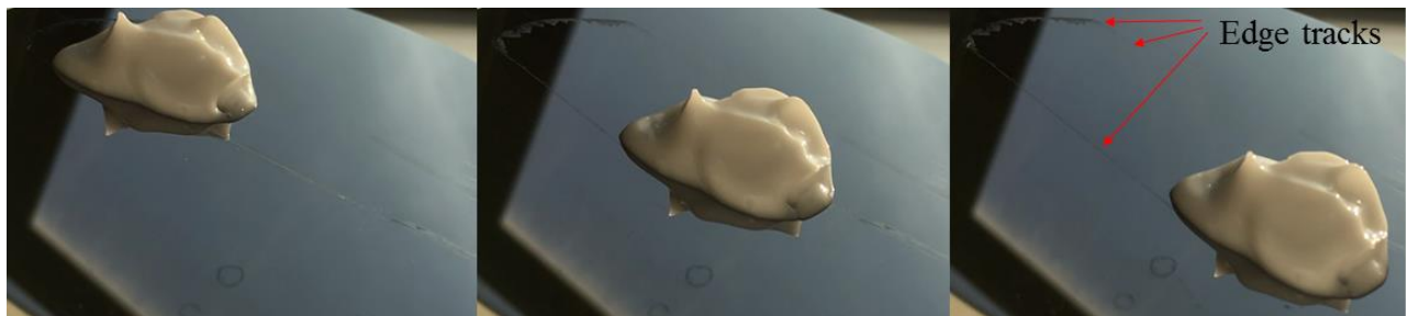
Figure 3: Successive views of a heap of emulsion (yield stress: 40 Pa) put on a smooth surface, at times: (a) 0, (b) 15.6 s, (c) 26 s. The sample length is about 3 cm. [Courtesy Xiao Zhang]
