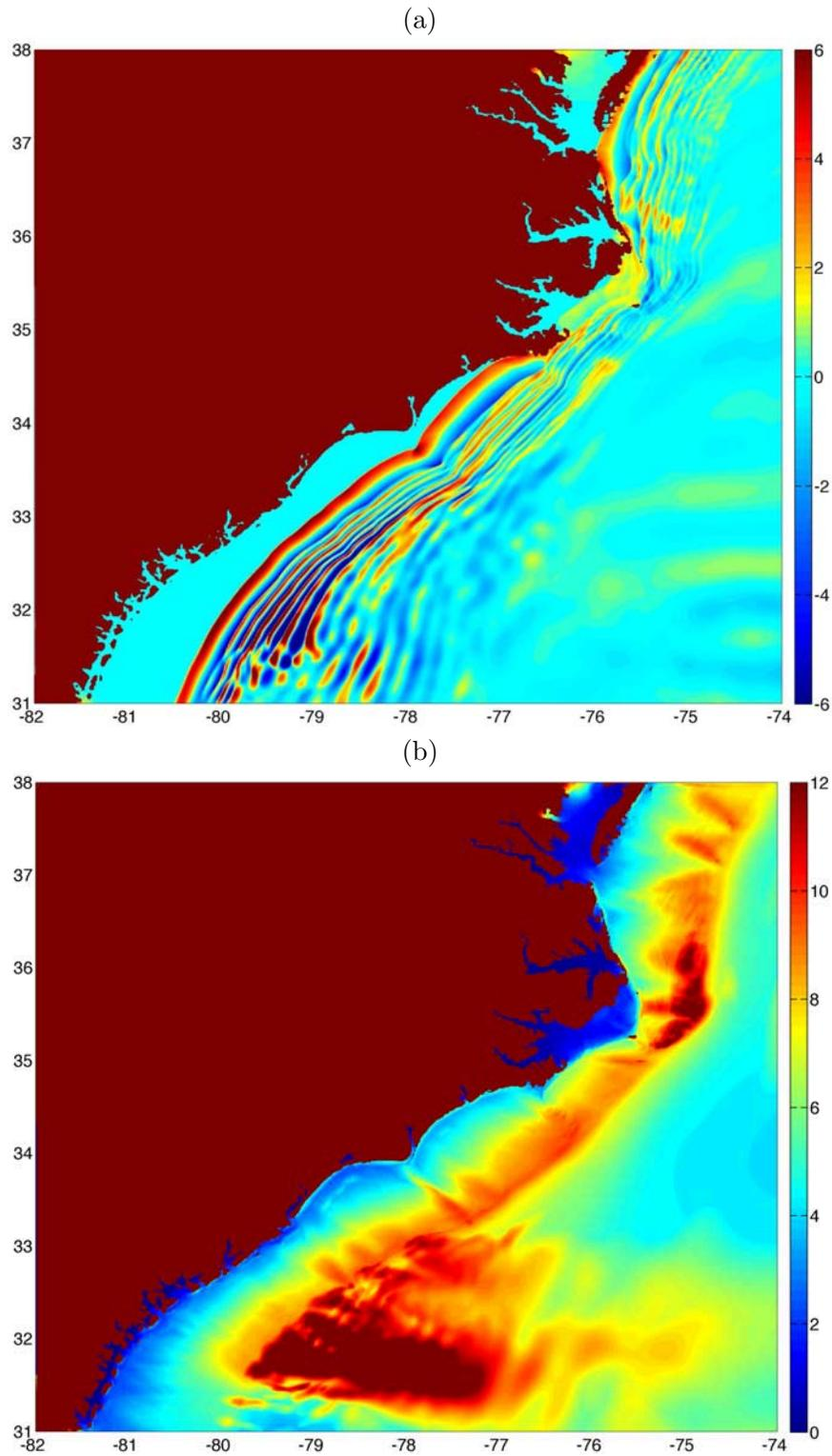
*Figure 12.* Surface elevation (color scale in meter) computed for the CVV 450 km<sup>3</sup> flank collapse scenario, in 20 arc-sec Mid US regional grid, off of South/North Carolina, Virginia, Maryland and Delaware (see Fig. 16 for locations of US states): (a) instantaneous elevation at 8h55'; and (b) maximum surface envelope up to 10h40', after the start of the event. Axes are Long. E. (deg.) and Long. N. (deg.).
