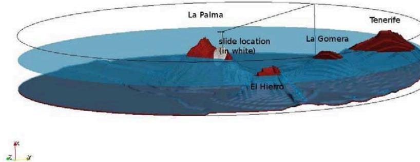
Figure 2. Sketch of THETIS 3D computational domain for the simulation of landslide tsunami generation. The white area in La Palma indicates the site of the  $80 \text{ km}^3$  subaerial slide. See Abadie et al. (2012) for details.
