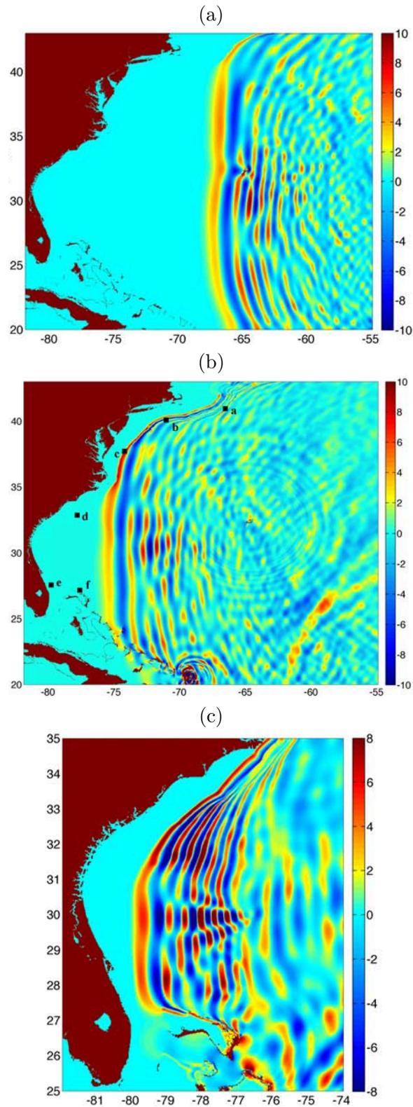
*Figure 7.* Surface elevation (color scale in meter) for the CVV 450 km<sup>3</sup> flank collapse scenario, computed with FUNWAVE-TVD in the 1 arc-min Atlantic ocean basin grid, at: (a) 6h20'; (b) 7h20'; and (c) 8h20', into the event. Axes are Long. E. (deg.) and Long. N. (deg.). Locations of stations a-f defined in Table II, with time series plotted in Fig. 8, are shown in (b).
