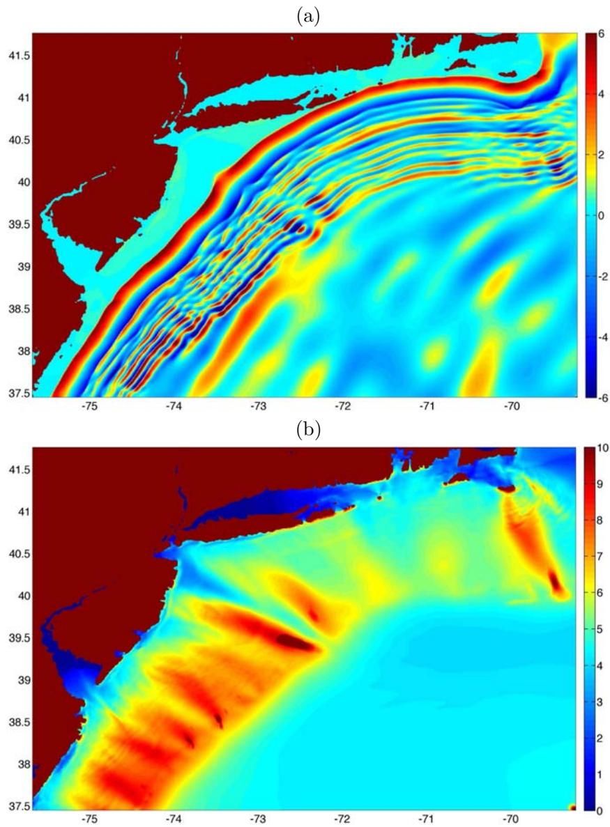
*Figure 11.* Surface elevation (color scale in meter) computed for the CVV 450 km<sup>3</sup> flank collapse scenario, in 20 arc-sec N. US regional grid, off of New Jersey, New York, and Massachusetts (see Fig. 16 for locations of US states): (a) instantaneous elevation at 8h10'; and (b) maximum surface envelope up to 9h30', after the start of the event. Axes are Long. E. (deg.) and Long. N. (deg.).
