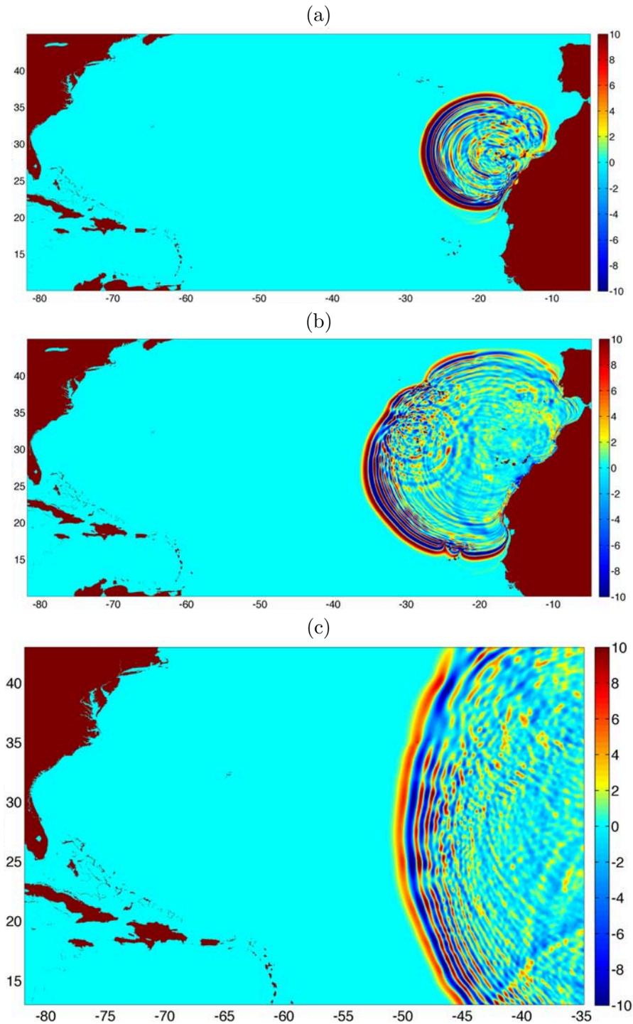
*Figure 6.* Surface elevation (color scale in meter) for the CVV 450 km<sup>3</sup> flank collapse scenario, computed with FUNWAVE-TVD in the 1 arc-min Atlantic ocean basin grid, at: (a) 1h20'; (b) 2h20'; and (c) 4h20', into the event. Axes are Long. E. (deg.) and Long. N. (deg.).
