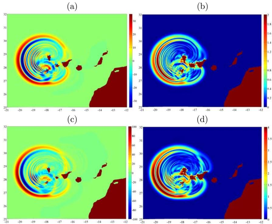
*Figure 5.* (a,c) Surface elevation (color scale in meter) and (b,d) horizontal water velocity magnitude (color scale in m/s) computed with FUNWAVE-TVD in the 500 m Cartesian grid defined in Fig. 1, at 20 min after the start of the CVV event, for Abadie et al.'s (2012): (a,b)  $450 \text{ km}^3$ ; and (c,d)  $80 \text{ km}^3$  flank collapse scenarios.
