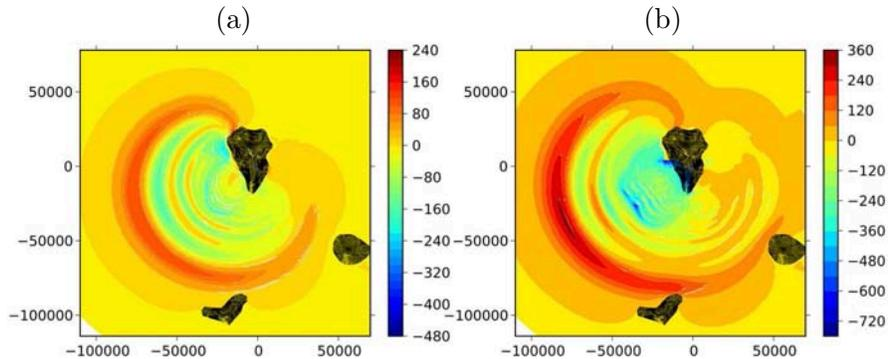
*Figure 3.* Surface elevations (color scale in meter) computed with THETIS for CVV flank collapse scenarios with volume: (a)  $80$ , (b)  $450 \text{ km}^3$ , at  $t = 7.5$  min after the start of the event. Note,  $x$  and  $y$  axes represent distance in meter.
