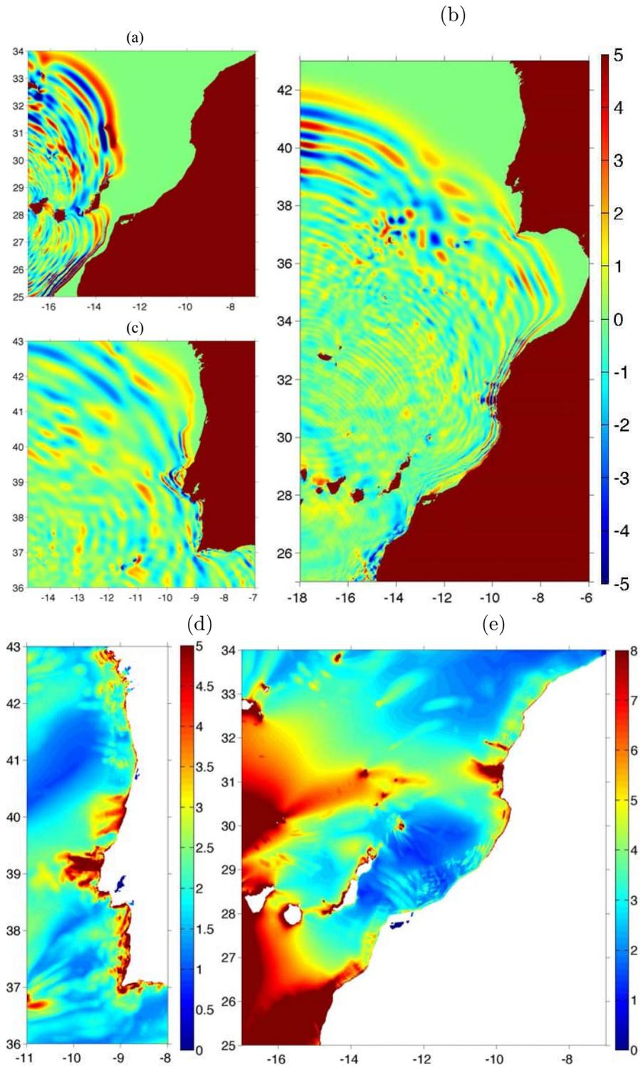
Figure 15. Surface elevation (color scale in meter) computed for the CVV 80 km<sup>3</sup> flank collapse scenario, in 15 arc-sec regional grid, off of western Africa and western Europe (Fig. 4, Table I). Instantaneous elevation at : (a) 1h20'; (b) 2h20'; and (c) 2h50'. Maximum surface envelope, up to 4h (d,e). Axes are Long. E. (deg.) and Long. N. (deg.).
