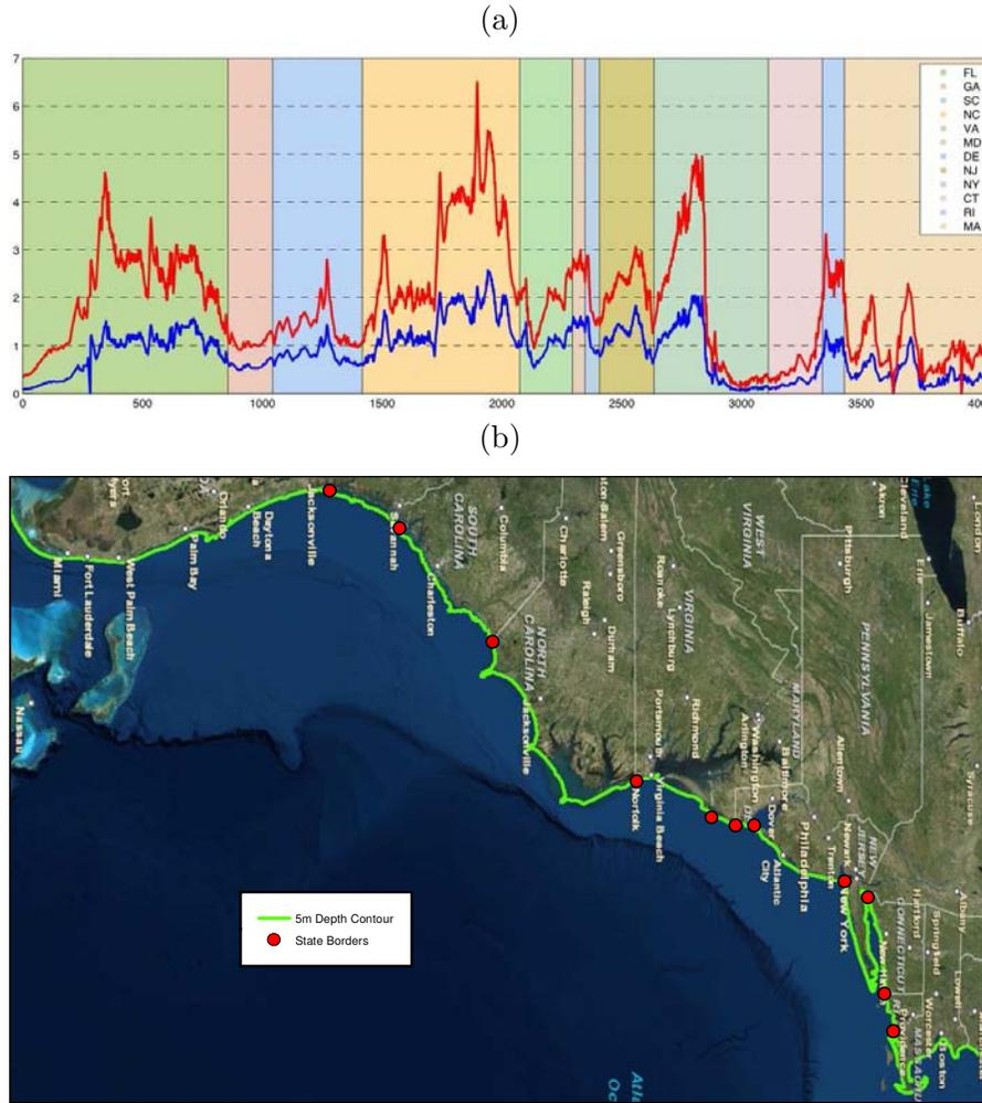
Figure 16. (a) Transects of maximum surface elevation (meter) computed for the 80 km<sup>3</sup> (blue) and 450 km<sup>3</sup> (red) scenarios, along a 5 m depth contour parallel to the US eastern coastline (show in (b)), as a function of the distance calculated along the contour (km), from south to north. Limits of the various US states are marked on both the transect (a) and the coastline (in (b)).
