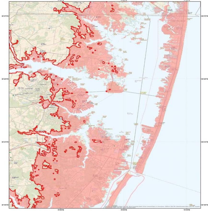
Figure 19. Tsunami inundation map (10 m resolution grid) for the 450 km<sup>3</sup> CVV flank collapse case (Abadie et al., 2012): inundation limit (thick red line); inundated area (pink area).
