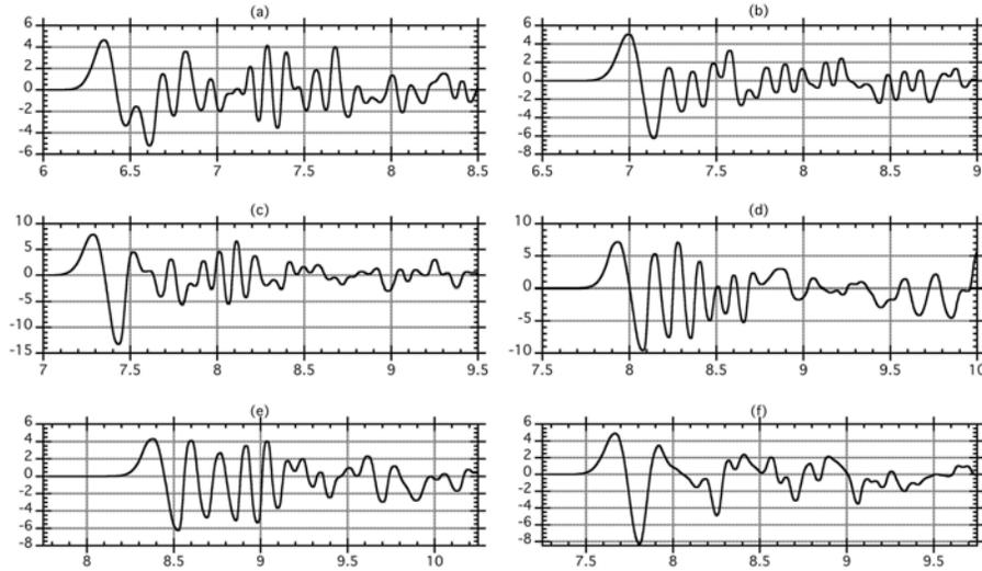
Figure 8. Time series of surface elevation ( $x$ -axis in hour and  $y$ -axis in meter) for the CVV 450 km<sup>3</sup> flank collapse scenario, computed at stations a-f (see Table II and Fig. 7b for location) with FUNWAVE-TVD, in the 1 arc-min Atlantic Ocean basin grid.
