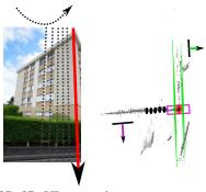
Figure 3: 2D-3D VL sweeping to extract secondary lines and planes (left). Top view of SfM point cloud (right) with regions to measure ridge cues (green), volumic points (red) and plane junctions (purple). Please see text for details.
