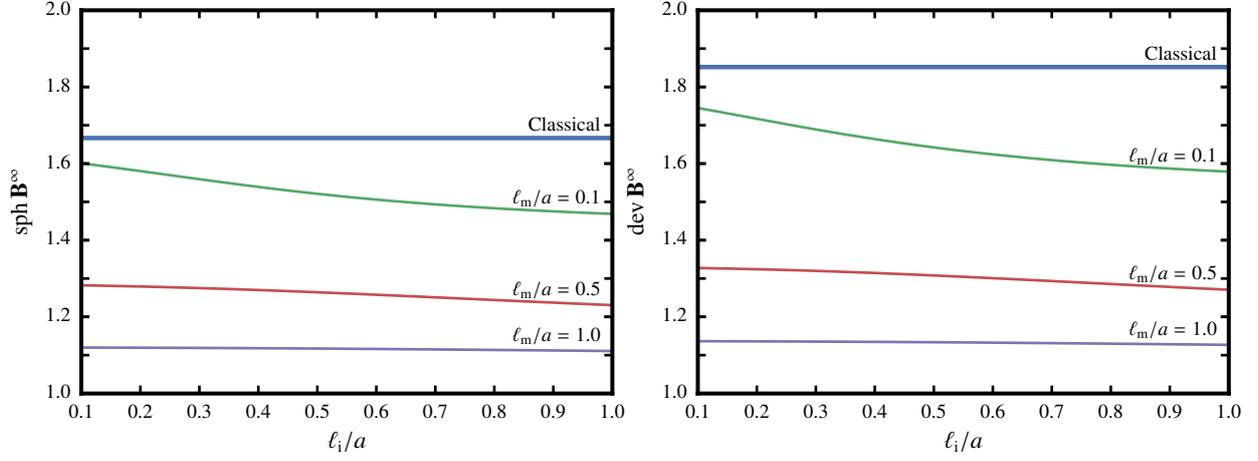
Figure 4: The spherical (*left*) and deviatoric (*right*) parts of the dilute stress concentration tensor  $\mathbf{B}^\infty$  as a function of the inhomogeneity's material internal length  $\ell_i$ . Like the previous graphs, colors correspond to various values of the material internal length  $\ell_m$  of the matrix. The thick line corresponds to the classical solution ( $\ell_i = \ell_m = 0$ ).
