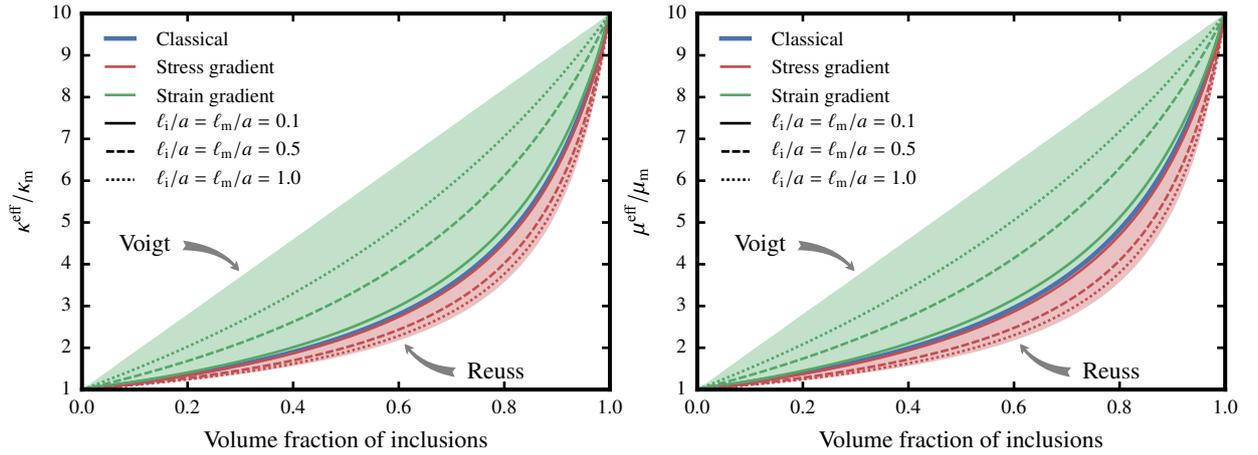
Figure 5: Mori–Tanaka estimates of the effective bulk (*left*) and shear (*right*) moduli of the composite  $\kappa^{\text{eff}}$  and  $\mu^{\text{eff}}$ , as a function of the volume fraction of inclusions,  $f$ . The estimates are represented for both stress- and strain-gradient materials.
