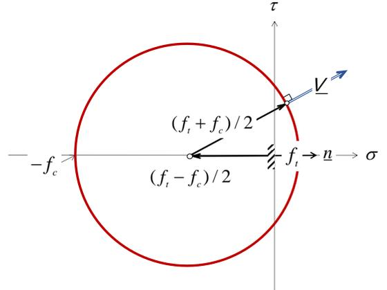
Figure 2. Rankine's intrinsic curve in the Mohr-plane
