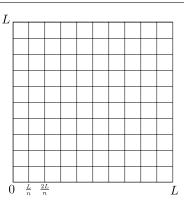
Fig. 2: Grid used for the discretization of the contact problem on the square surface  $\Omega = [0; L] \times [0; L]$
