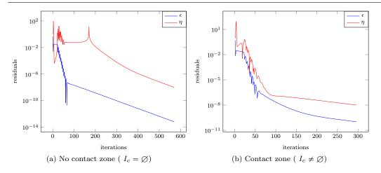
Fig. 5: Residuals  $\eta$  and  $\epsilon$  versus iterations of the proximal algorithm for the two imposed displacements  $u_0 = 1.302L$  and  $u_0 = 1.2L$
