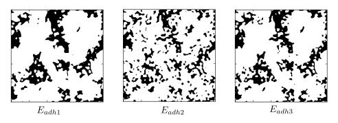
Fig. 8: Equilibrium solution : gap obtained for the three adhesive potentials: black means contact, white means no contact.
