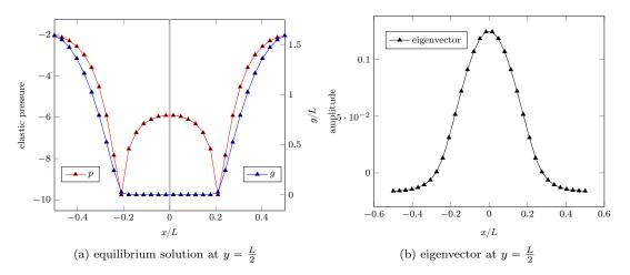
Fig. 4: Hertz case: equilibrium solution for imposed displacement  $u_0 = 1.2L$  (solution with a contact zone) and instability mode associated to  $\lambda_{min} = -4.55$
