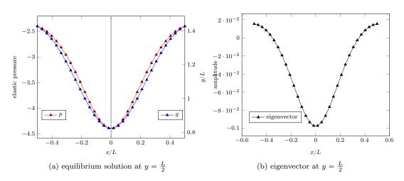
Fig. 3: Hertz case: equilibrium solution for imposed displacement  $u_0 = +1.302L$  (solution without contact) and instability mode associated to  $\lambda_{min} = -7.3 \ 10^{-6}$
