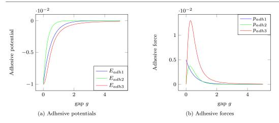
Fig. 7: Graphical representation of the three adhesive potentials and associated forces
