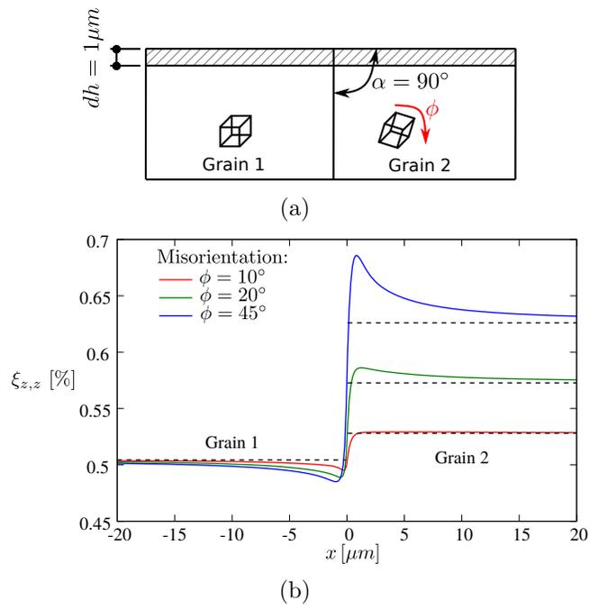
Figure 6: (a) Schematic representation, (b) and simulated displacement gradient component  $\xi_{z,z}$  profiles (solid lines) for three different misorientations  $\phi$  of Grain 2. The dashed lines represent the semi-analytical grain independent model.
