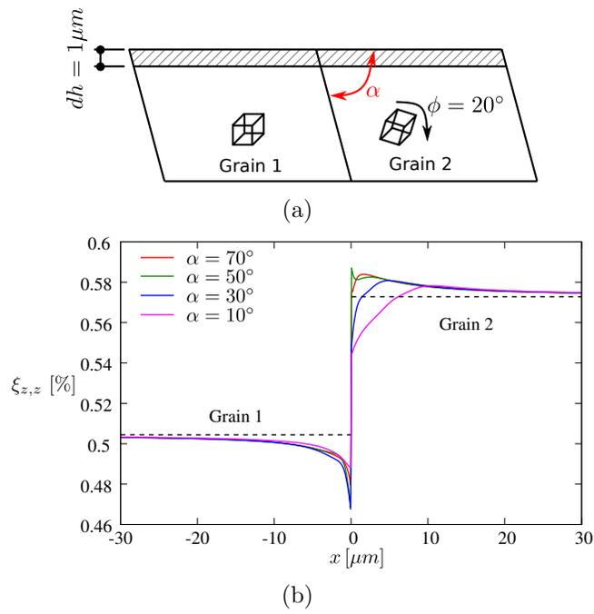
Figure 7: (a) Schematic representation, (b) and simulated displacement gradient component  $\xi_{z,z}$  profiles (solid lines) for four different grain boundary orientations  $\alpha$ . The dashed lines represent the semi-analytical grain independent model.
