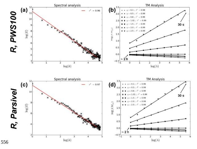
557Figure 2: Scaling analysis for *R* measured by the PWS100: (a) Spectral analysis, i.e. equation 55814 in log-log plot; (b) Trace Moment (TM) analysis, i.e. equation 9 in log-log plot. (c) and (d) 559Same as (a) and (b) for *R* measured by the Parsivel<sup>2</sup>.
