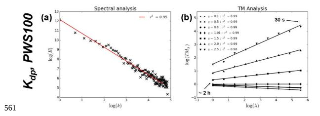
562Figure 3: Scaling analysis for  $K_{dp}$  measured by the PWS100: (a) Spectral analysis, i.e. 563equation 14 in log-log plot; (b) Trace Moment (TM) analysis, i.e. equation 9 in log-log plot 564
