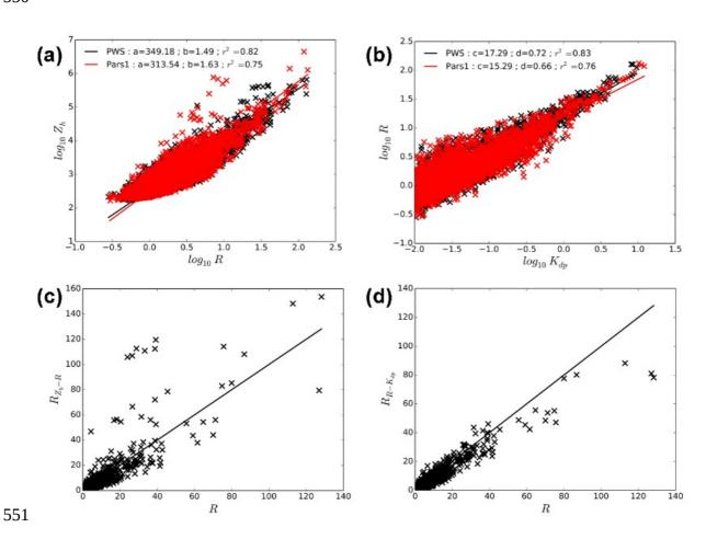
552Figure 1: Computation of the parameters of the  $Z_h - R$  (a) and  $R - K_{dp}$  (b) relations 553(equations 16 and 17 respectively in log-log plot). Scatter plot of  $R_{Z-R}$  (c) and  $R_{R-K_{dp}}$  (d) 554versus R for the PWS100 data
