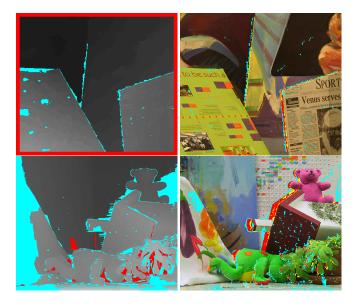
**Fig. 2**. Disparity map (left) and occlusion map (right). Left: in red, the unknown disparity value and in cyan, the estimation error. Right: in red, the true positive, in yellow, the false negative and in cyan, the false positive.
