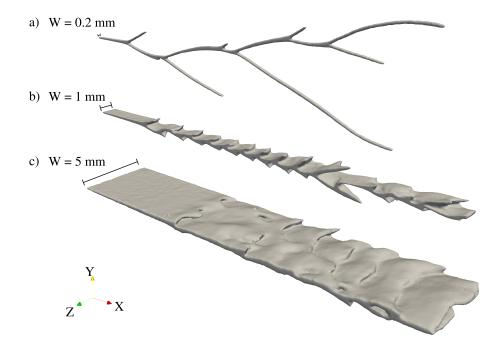
Many aspects of the microbranching instability [1] are not fully understood such as the difference of crack patterns observed in PMMA on one hand and glass or brittle gels on the other hand [2]. In this work, we simulate the microbranching instability of fast propagating cracks using a variational phase-field approach and show that three-dimensional effects are fundamental for understanding the origin of this instability.
