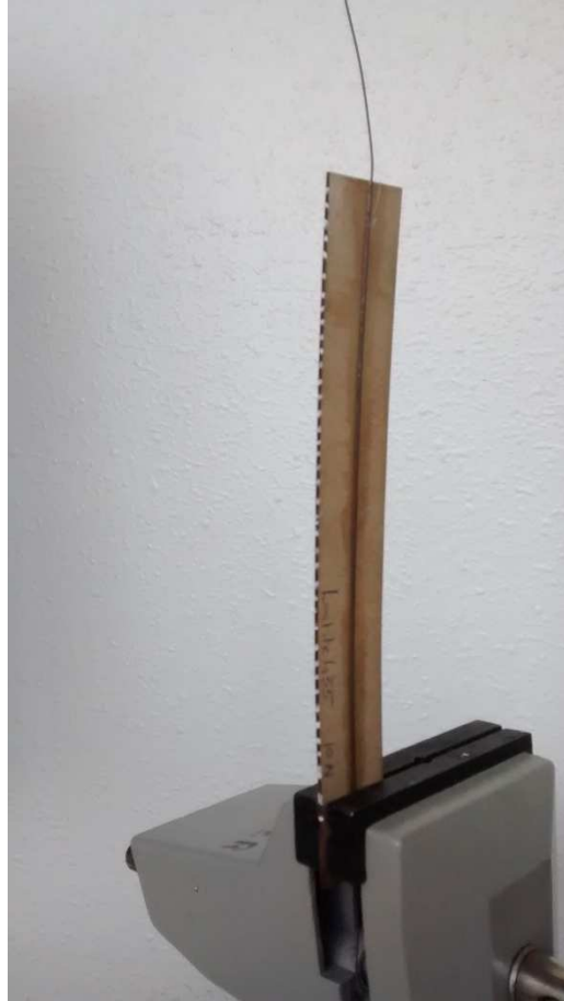
Fig. 1. Bilayer-type actuator composed of a wooden lamella and an SMA wire: initial state at ambient temperature
