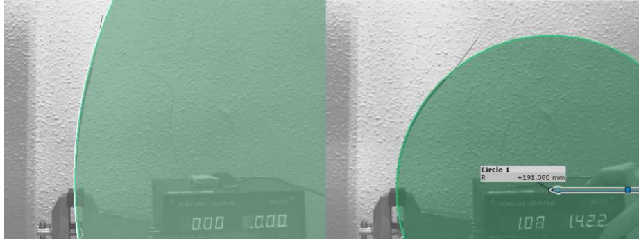
Fig. 2. Curvature measurements for the bilayer-type actuator: initial state at ambient temperature (left), actuated state with resistive heating (right)
