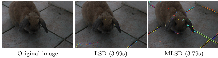
Fig. 7: Lines detected with LSD [2] (middle) and with MLSD [3] (right) in a 15 Mpixels image (left).
