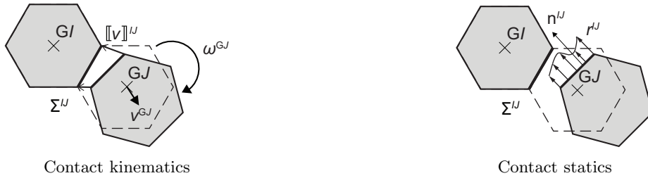
Figure 4: Kinematics and statics of the contact model adopted for the discrete medium.
