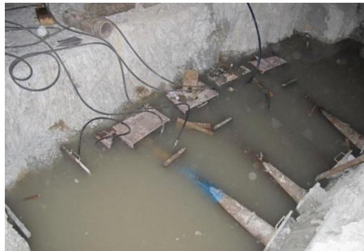
Figure 2. Field test on thin-layer rock masses in water soaked condition.
