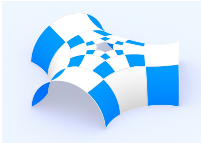
Figure 10: The result of the hole filling strategy, with smooth T-joints between patches.
