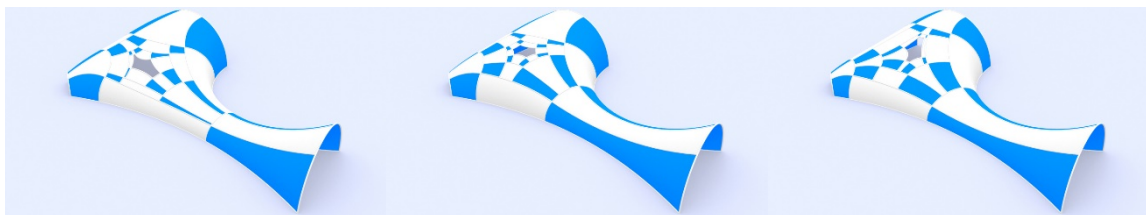
Figure 15: Several solutions obtained with the hole-filling problem for an irregular hole. Values of E_2 , from left to right: 38.7, 36.5, 38.2
