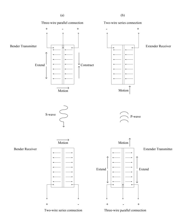
Figure 1. Sketch of bender and extender connection: (a) transmitting S-wave; (b) transmitting P-wave (after Lings and Greening 2001)
