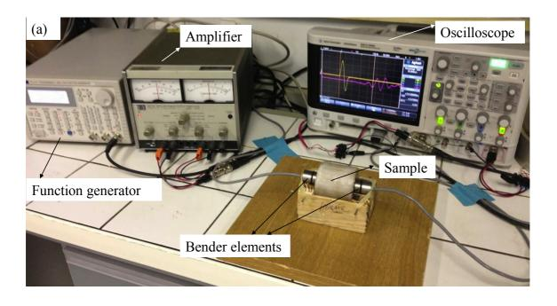
Figure 4. Setup of the bender element testing: (a) photo of the setup; (b) schematic diagram of the setup
