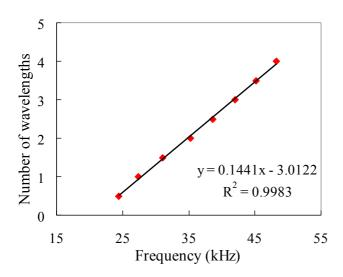
Figure 6. Measurements by " $\pi$ -point" method on a lime-treated soil (D1)
