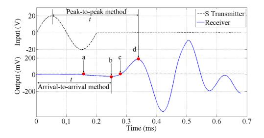
Figure 2. Typical S-wave transmitted and received signals
