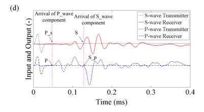
Figure 7. Determination of the arrival point by S+P method on a lime-treated soil (D1): (a) f = 20 kHz; (b) f = 30 kHz; (c) f = 40 kHz; (d) f = 50 kHz
