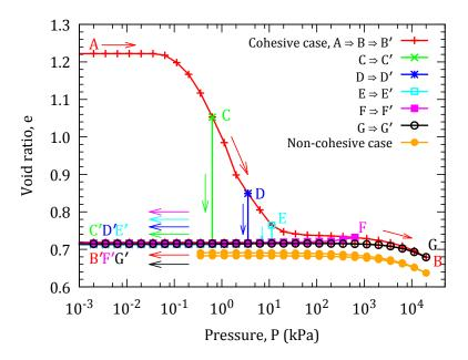
FIG. 5. Void ratio versus reduced pressure  $P^*$ , as cohesive forces are suppressed at the beginning of unloading, starting at different points on the primary compression curve. (In this case the initial state had solid fraction  $\Phi_0=0.45$ ).
