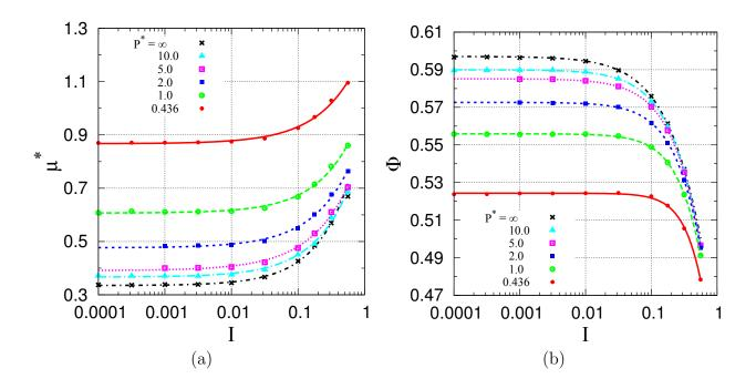
FIG. 6. (a) Internal friction coefficient  $\mu^*$  and (b) solid fraction  $\Phi$  versus I for different values of  $P^*$ .
