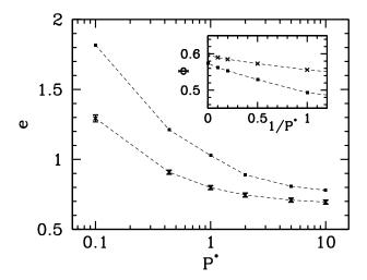
FIG. 7. Main plot: void ratios in primary isotropic compression,  $e_{\rm iso}$  (square dots), and in critical state,  $e_0$  (crosses with error bars) versus  $\log P^*$ . Inset: detail of variations of solid fraction  $\Phi_{\rm iso}$  in isotropic compression (square dots), and  $\Phi_0$ , in critical state (crosses), for large  $P^*$  (including the dry case of infinite  $P^*$ ), versus  $1/P^*$ . Dashed lines are drawn to guide the eye.
