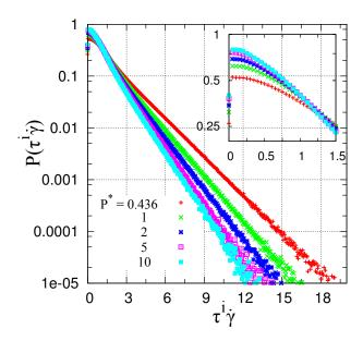
FIG. 10. Distribution of the age of menisci for different  $P^*$  values (results for different I indistinguishable on this plot). Inset shows detail of initial decay.
