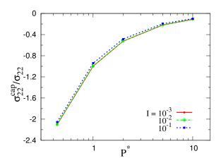
FIG. 9. Contribution of capillary forces to normal stress  $\sigma_{22}$ .
