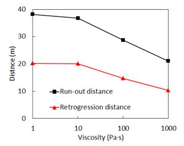
Figure 21. Curves of run-out distance and retrogression distance against viscosity
