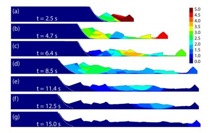
Figure 19. Velocity contour during the retrogressive failure
