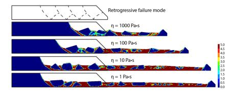
Figure 20. Final deposits from the simulation using different viscosity coefficients for sensitive clays
