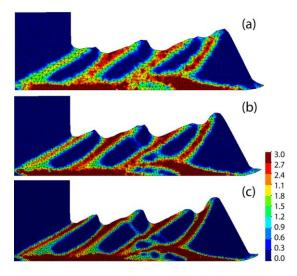
Figure 15. Final configurations and shear band distributions of the column collapse using (a) coarse meshes, (b) medium meshes, and (c) fine meshes. Colours are proportional to the accumulated equivalent plastic strain
