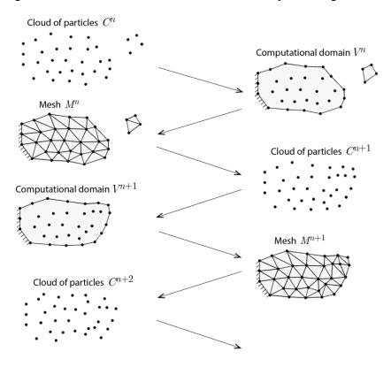
Figure 4. Steps for the Particle Finite Element Method (after [35])
