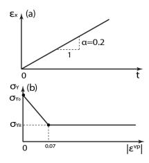
Figure 8. Curves of (a) the applied strain rate and (b) the variation of the yield stress for the one-dimensional strain-softening problem
