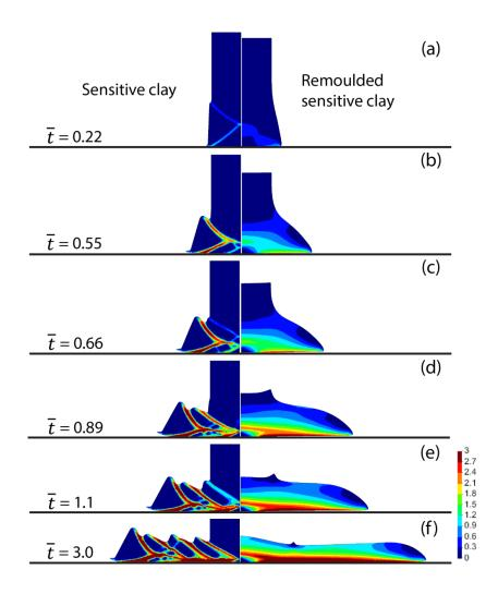
Figure 11. Collapse evolution processes of the column of initially undisturbed sensitive clays and remoulded sensitive clays. Colours are proportional to accumulated equivalent plastic strain
