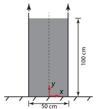
Figure 10. Schematic diagram for the collapse of a column of sensitive clays
