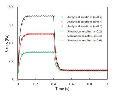
Figure 7. Comparison of numerical and analytical solutions for the one-dimensional stress relaxation problem
