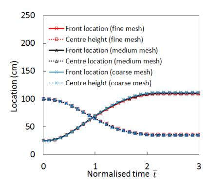
Figure 14. Effects of the utilized mesh size on the curves for front location and centre height of the column against normalized time
