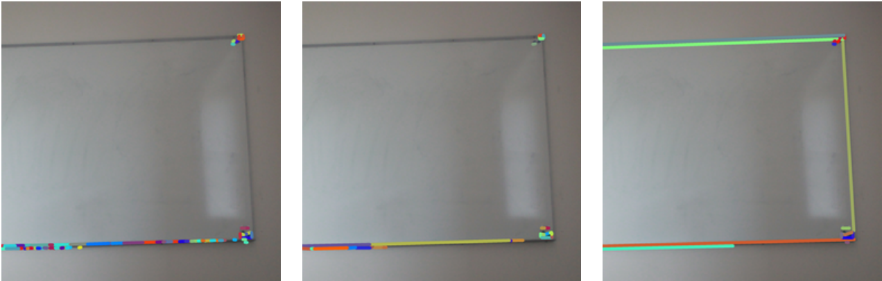
Fig. 3: From left to right: detection upon a low contrast area for LSD [6], EDLines [1] and our method. Notice that our method does not suffer from over-segmentation and that upper and lateral borders of the white board are detected.
