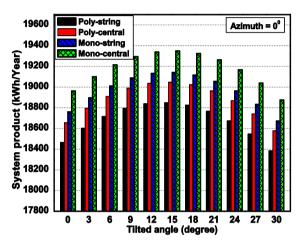
Fig. 6. System product of PV system for  $A_m = 0^0$  by tilted angles
