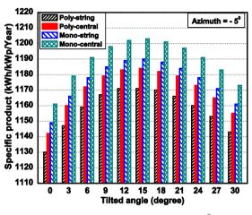
Fig. 10. Specific product of PV system in zone 1,  $A_m = -5^0$  by tilted angles
