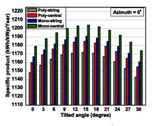
Fig. 5. Specific product of PV system for  $A_m = 0^0$  by tilted angles
