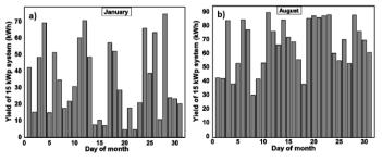
Fig. 9. Average daily yield of 15 kWp PV array for January and August.
