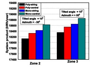
Fig. 12. Specific product of PV system in zone 2 and 3 with  $\theta_{\rm m} = 15^{\circ}$
