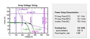
Fig. 4. PV Array sizing in PVSYST [9], 12 XL SW 335 poly-crystalline modules in series and 4 strings, using Ingecon Sun 15 TL M inverter
