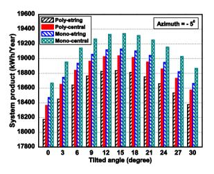
Fig. 11. System product of PV system in zone 1,  $A_m = -5^0$  by tilted angles
