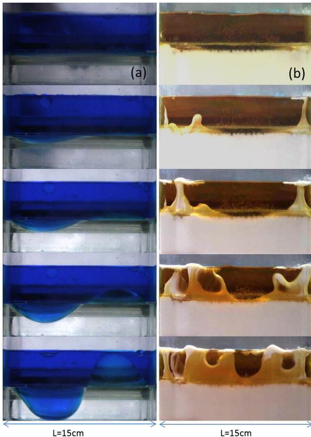
FIG. 1. RTI development for (a) viscous Newtonian fluid (Silicone oil, 0.35 Pa.s viscosity) initially below a denser colored water-ethanol solution ( $\Delta\rho/\rho = 1.3\%$ ) at times (from top to bottom): 0 (midtime of gate opening), 6, 12, 18, and 24 s; and (b) a concentrated (white) emulsion ( $\tau_c = 9.6$  Pa) initially below a (brown) denser salt solution ( $\Delta\rho = 600$  kg m<sup>-3</sup>) at times: 0, 1.9, 3, 3.8, and 4.5 s.
