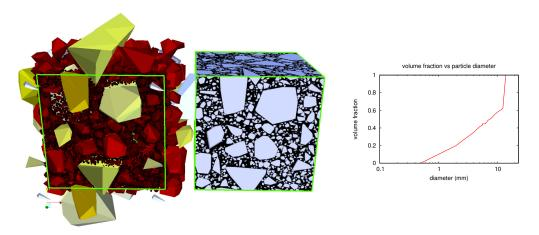
Figure 3: A 4 cm-wide sample of a concrete made of coarse sand (d > 0.5 mm) and small gravel (d < 13.5 mm) built by the RSA algorithm is shown along with its discretation on a  $384 \times 384$  grid. The volume fraction of polyhedral inclusions in the cubic cell is 60%.
