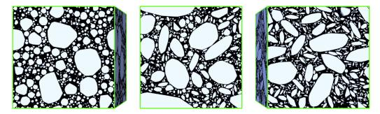
Figure 7: Microstructures featuring spherical (a/b = 1), elongated (a/b = 3) or flat (a/b = 0, 33) aggregates are discretized on  $384 \times 384 \times 384$  regular grids to perform full 3D numerical simulations. The volume fraction of aggregates is 60%.
