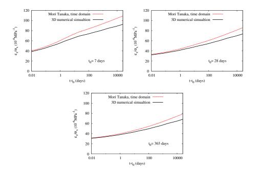
Figure 5: The normalized creep strains  $\varepsilon_x/\sigma_x$  of a concrete estimated by the time-space method of Sanahuja [81] and full 3D numerical simulations are displayed as functions of the time elapsed since loading  $t - t_0$ . Considered times of loading are  $t_0 = 7$  days (top left),  $t_0 = 28$  days (top right) and  $t_0 = 365$  days (bottom). The inclusions are assumed to be spherical so as to use the model of Sanahuja. The loading corresponds to an uniaxial creep test.
