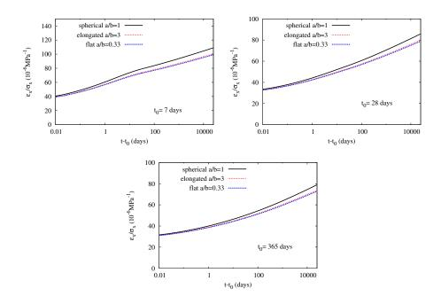
Figure 6: The estimated normalized creep strains  $\varepsilon_x/\sigma_x$  of concrete featuring different aspect ratios of aggregates are displayed as functions of the time elapsed since loading  $t-t_0$ . Considered time of loading are  $t_0 = 7$  days (top left),  $t_0 = 28$  days (top right) and  $t_0 = 365$  days (bottom). In case of uniaxial creep tests, the aspect ratio of aggregates has little effect on the time-dependent strains of concretes estimated by the time-space method.
