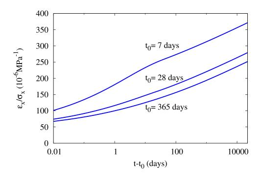
Figure 4: The normalized creep strains  $\varepsilon_x/\sigma_x$  of a cement paste according to the modified B3 model [8] are displayed as functions of the time elapsed since loading  $t - t_0$  for different times of loading  $t_0$ . An uniaxial creep test  $\sigma_x$  is considered. The Young modulus  $(t - t_0 \approx 0.01 \text{ days})$  depends on the time of loading  $t_0$ . The long term trend of creep strains is logarithmic  $(t - t_0 \ge 100 \text{ days})$ .
