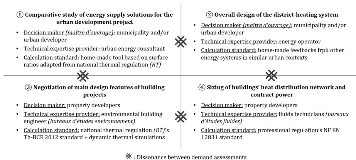
**Figure 5.** At each of the four steps in the DH design process, heat demand is estimated by a different actor using a new calculation standard, which leads to dissonances between the various demand assessments.
