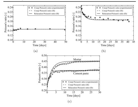
Fig. 5 Experimental data of multiaxial creep experiments on cementitious materials: (a) Biaxial creep test on cubic concrete sample (Jordaan and Illson 1969); (b) Uniaxial creep test on a cuboid sample of cement paste (Parrott 1974); (c) Triaxial creep tests on cylindrical specimens of leached cement paste and mortar (Bernard et al. 2003)
