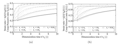
**Fig. 6** Ratio  $-\varepsilon_l(t)/\varepsilon_a(t)$  of the lateral to the axial strain (*black lines*) observed during creep experiments with various durations  $\tau_L$  of the loading phase, and creep Poisson's ratio  $\nu_c$  (*gray lines*) for a material that creeps deviatorically and whose deviatoric creep behavior is modeled by (**a**) the Maxwell unit or (**b**) the Kelvin–Voigt unit
