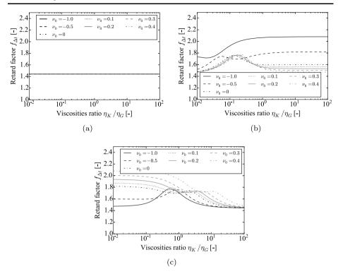
Fig. 4 Retard factor  $f_{\Delta t}$  of the creep Poisson's ratio  $v_c(t)$  with respect to the relaxation Poisson's  $v_r(t)$ : (a) Both volumetric and deviatoric behaviors governed by the Maxwell unit (see Fig. 1a); (b) Volumetric behavior and deviatoric behavior governed by the Maxwell unit and the Kelvin–Voigt unit, respectively (see Fig. 1b); (c) Volumetric behavior and deviatoric behavior governed by the Kelvin–Voigt unit and the Maxwell unit, respectively (see Fig. 1c)
