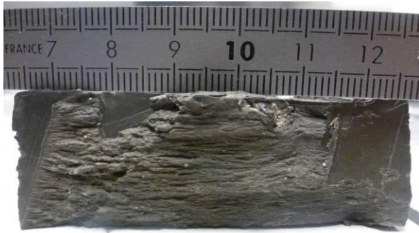
601 602 Figure 5: Bedding plane on natural Boom Clay sample.
