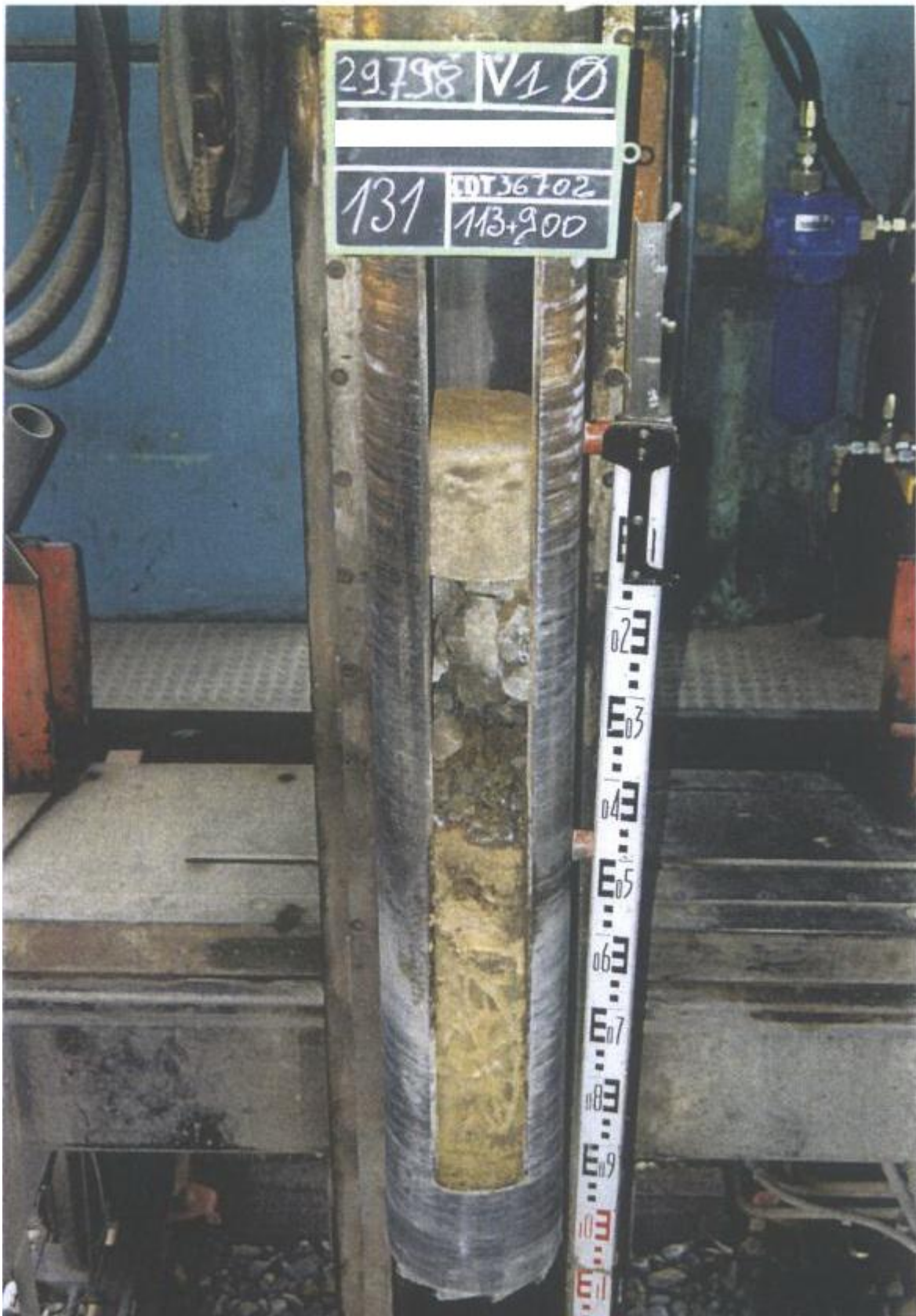
Fig. 10: Core sample from typical conventional railway sub-structure
