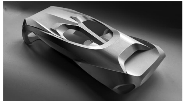
Figure 13. A developable car model designed by Kyungeun Ko for Bentley ™ and prototyped by Robofold ® [41].
