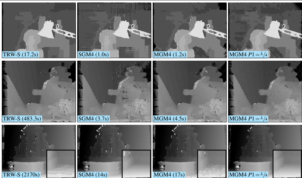
Figure 3: Qualitative result comparison for the images Tsukuba and Teddy from [22], plus a low resolution Fountain from [23]. Note that in the result of MGM4 there are no streaking artifacts as in the baseline SGM4. The last column (MGM4 P1 = \lambda/4 ) and the detail magnified in the last figure are commented in the text.
