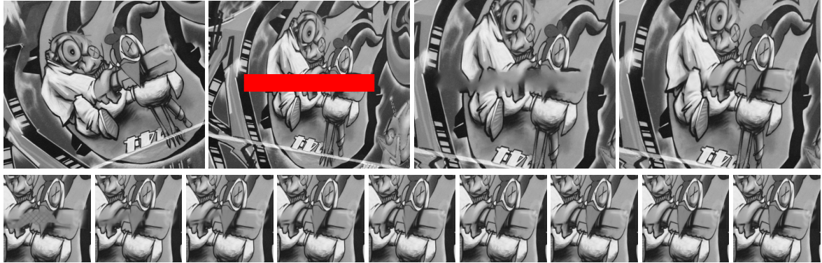
Figure 7: First row: source image, target image with the inpainting domain shown in red, and close-ups around the inpainting area of the NL-Means result and the result of our method. Second row: evolution of the inpainting domain over iterations of our method (every third iteration).
