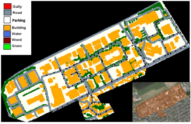
Figure 4: Map of the land use distribution inputted in Multi-Hydro for the Loup catchment with pixels of size 10 m x 10 m. The sewer network modelled with SWMM is superposed to this map (the nodes and conduits are visible along most of the roads). Satellite image the catchment (lower right)
