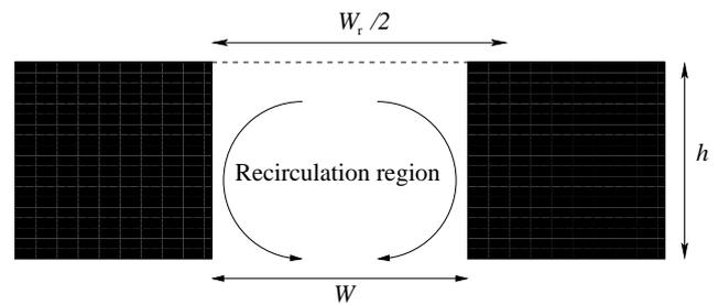
**Figure 1.** Narrow canyon leading to a skimming flow.
