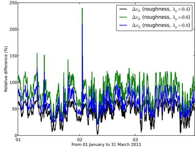
**Figure 11.** Time series of dry deposition velocity relative difference between the urban canopy and roughness-length models from January 2011 to March 2011 in one chosen urban grid cell for three values of the building density.
