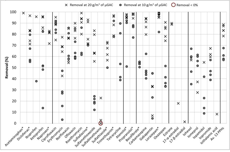
Figure 3 - Removals of PPHs (n = 31) by  $\mu GAC$  treatment in stabilized phase at 10 and 20  $g_{\mu GAC}/m^3$
