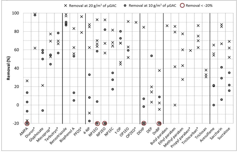
Figure 4 - Removals of the other emerging pollutants within  $\mu GAC$  treatment
