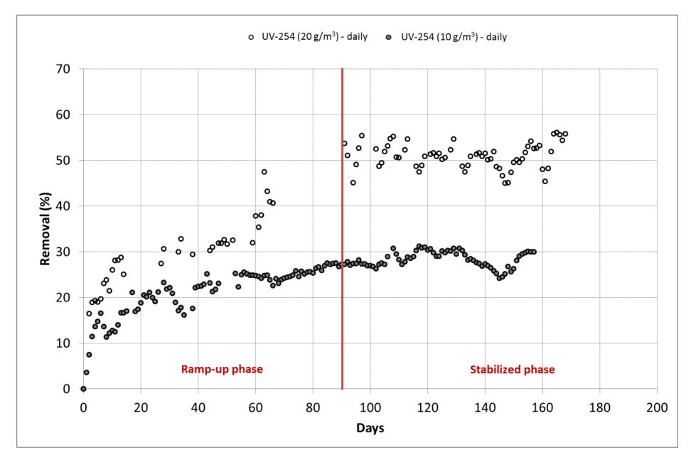
Figure 2 - Ramp-up phase of the CarboPlus® process for both assessed doses (10 and 20  $g_{\mu \rm GAC}/m^3$ )
