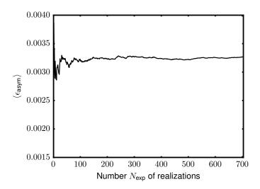
Fig. 3. Convergence of the statistical estimator for the mean field of  $\{\epsilon_{asym}(\mathbf{x},\theta), \mathbf{x} \in \Omega\}$  at the center of domain  $\Omega$ .
