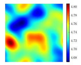
**Fig. 5.** Plot of mean function  $(x_2, x_3) \mapsto \mu_{\mathrm{m}}^{-1} \langle \tilde{C}_{1111}(L/2, x_2, x_3) \rangle$ .
