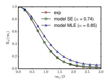
Fig. 13. Estimated covariance function of the random bulk modulus along the  $x_1$ -axis: comparison between experimental data and model-based simulations.
