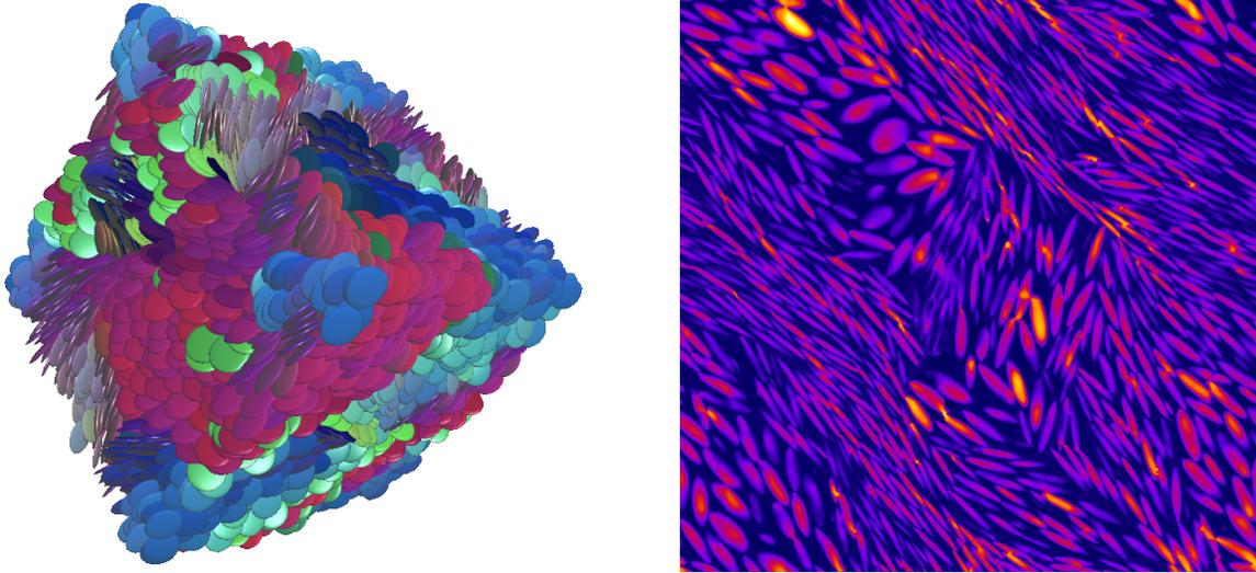
**Figure 1.** The microstructure to be homogenized (left, reproduced from [Brisard and Levitz, 2013](#)), and a 2D cut through the 3D map of  $\tau_{12}$  (right), for a macroscopic strain  $\mathbf{E} = \mathbf{e}_1 \otimes \mathbf{e}_2 + \mathbf{e}_2 \otimes \mathbf{e}_1$ . On  $1024^3$  grids, the method reveals fine details of the mechanical fields.
